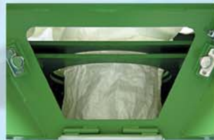
'Drop-stop' to tie off and remove partially emptied Big-Bags
