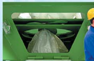
'Drop-stop' to tie off and remove partially emptied Big-Bags
