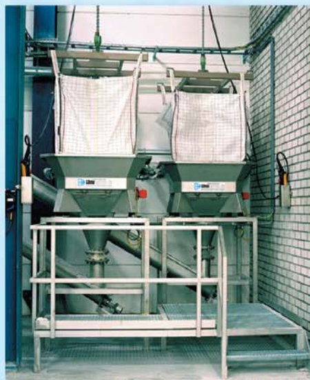
Big-Bag discharger Model LB2 with rigging frame, outlet spout and screw conveyor
